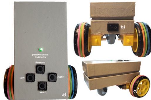
Figure 2. The Robo-1 model developed on the base of the Arduino platform: a) top view with indicated control knobs and performance indicator; b) back view with the switch on-off knob; c) general view of the robot.
